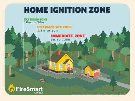
Immediate Zone (Om - 1.5m): Remove all ignitable material adjacent to home. Refurbish structure to reduce flammability. Prevent embers from igniting structure. Noncombustible surface should extend around the entire home and any attachments.
